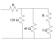
The three branches in parallel have an equivalent resistance of:
